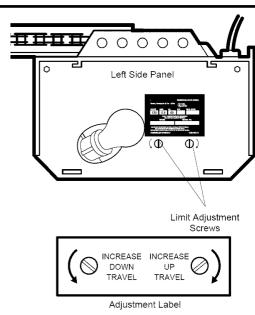
Adjustment procedures are outlined below. Run the opener through a complete travel cycle after each adjustment.
